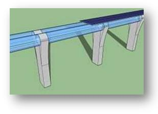
capsule floats on a 0.02-0.05 in (0.5-1.3 mm) layer of air provided under pressure to air-caster "skis", similar to how pucks are levitated above an air hockey table, while still allowing faster speeds than wheels can sustain. Hyperloop One's technology passive maglev for the same uses purpose. Linear induction motors located along the tube would accelerate and decelerate the capsule to the appropriate speed for each section of the tube route. With rolling
