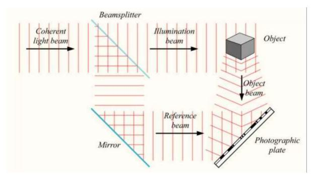
To create a hologram, you need an object (or person) that you want to record; a laser beam to be shined upon the object and the recording medium; a recording medium with the proper materials needed to help clarify the image; and a clear environment to enable the light beams to intersect.
